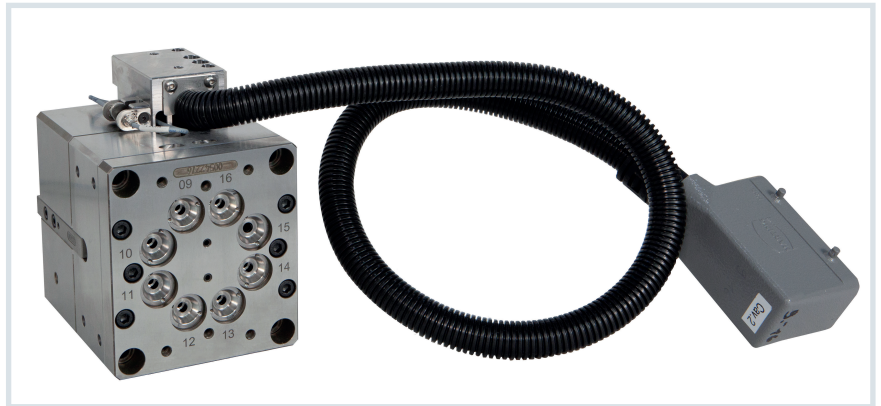
Fig. 3. Replaceable mold insert: cluster for eight pipette tips with own electrical supply for the individually heated nozzle tips © Männer
