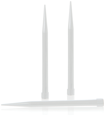
Fig. 1. Polypropylene pipette tips. The wall thickness is 0.3 mm, the diameter of the suction opening is 0.35 mm © Männer
